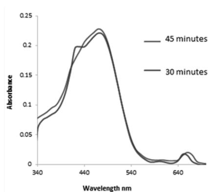
**Fig. 6.** UV-Vis absorption spectra of astaxanthin extracted by ultrasound pretreatment at 30 and 45 minutes
