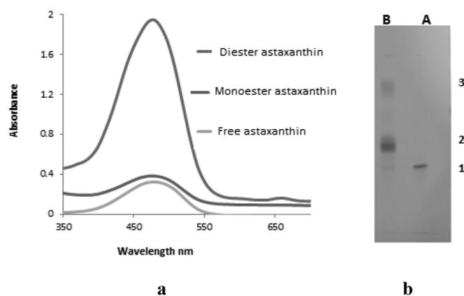
**Fig. 10.** a) Isolation of astaxanthin forms by TLC: A sample of standard astaxanthin, B substance extracted from *H. pulvialis*, b) Absorption spectrum of astaxanthin and monoester and diester derivatives isolated by TLC
