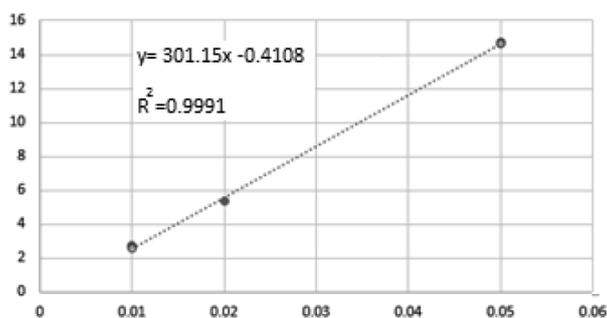
**Fig. 12.** Standard curve for astaxanthin by HPLC
