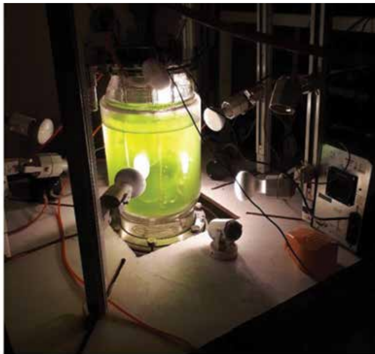
Fig. 1. A photobioreactor, with a volume of 10 liters, illuminated by four artificial light sources and continuously aerated with filtered air
