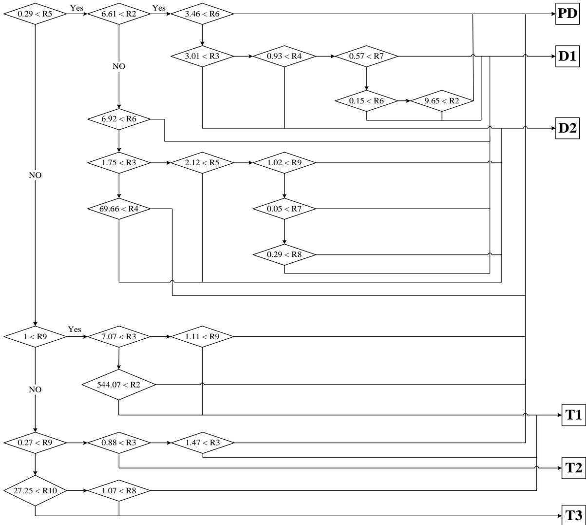
Fig. 7. NGR method to detect incipient faults in oil immersed transformers.
