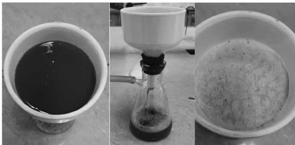
Fig. 2. Removing cell debris via filter paper
